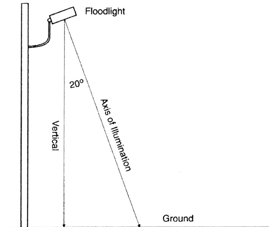
Exhibit 1. See *An Ordinance to Improve Outdoor Lighting in the City of Alpine, Texas, Section 3 (A) 1*: For spotlights and floodlights mounted overhead on poles and used for area lighting, the axis of illumination shall be adjusted to an angle not more than 20 degrees from the vertical line between the fixture and the ground.
